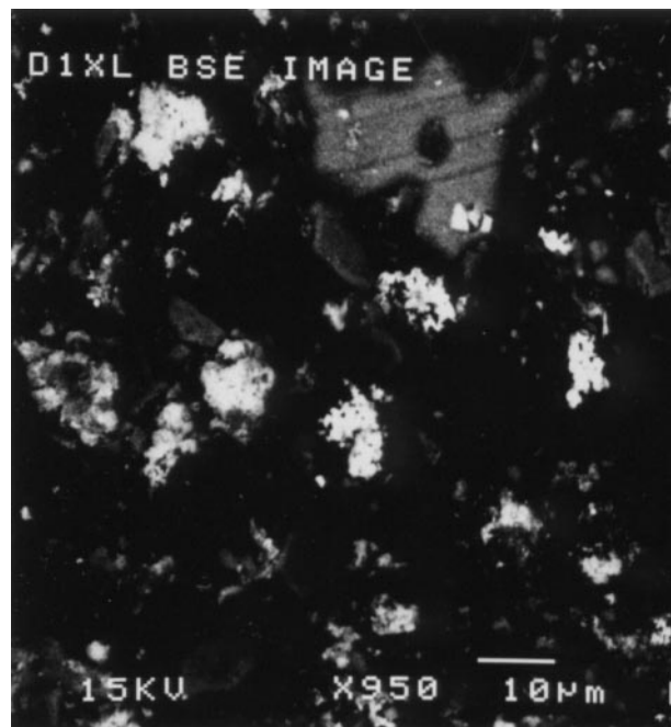
Fig. 6 SEM backscatter image of particles collected near the outlet to cell 2, approximately 4 ft below the surface. The bright spots have a higher mean atomic mass, and are mostly ZnS particles. The darker regions are a mix of organic and mineral matter inherited from the cell substrates.
